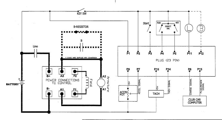
NOTE: B-RESISTER AND CONTACTOR ARE OPTIONAL ON SOME MODELS AND ARE NOT NEEDED WITH **UPGRADE**
