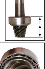
DV: On face of pinion gear
