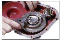
Idler Gear Circlip
