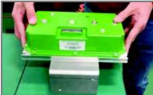
Mounting plate with controller fastened in place.
