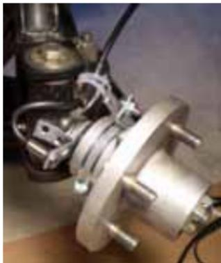
Secure the cable with cable clamps. Watch for CHAFFING points that may damage the cable. Always use TWO cable ties side by side (should one break in the future)
