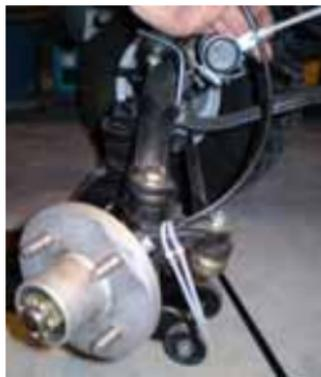
Feed the connector over the TOP of the steering column. Let cable hang for now. (as shown in the Temp Extension Cable Installation section)
