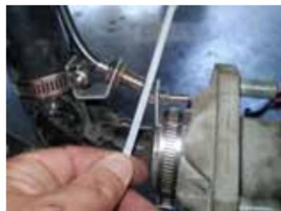
**SLOWLY** rotate the wheel hub and check for any interference that could damage the 6mm magnet.
