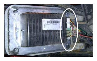
3. Carefully unplug all connections to the factory controller and remove the three – 13mm bolts securing the four large diameter wires. Save these bolts they will be reused when installing the new controller.
