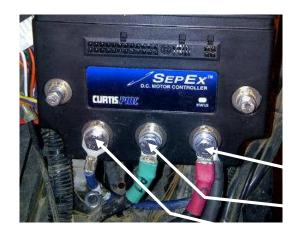
1. Using the three 13mm bolts retained when the original controller was removed, securely fasten the four large diameter wires to the new controller.
