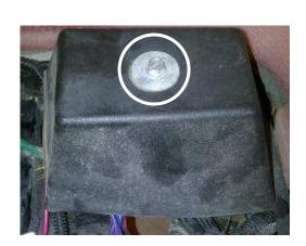
**7.** Remove the solenoid environmental protection cover.
