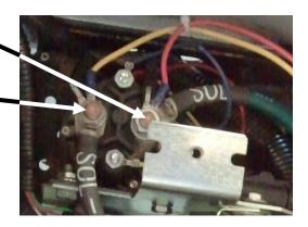
**11.** Plug the two wire- four pin walk-away harness connector to the two wire- four pin conversion harness connector then re-install solenoid cover using original hardware.
