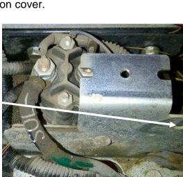
**8.** We will be using an open hole on the solenoid cover mounting tab to fasten the walk-away relay and protection fuse.
