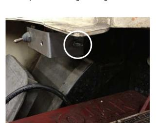
**14.** Mount the new tow/run switch mounting plate using an open hole in the vehicle frame right above the new controller using the included M6x25mm bolt, washer, lock washer, and nut.
