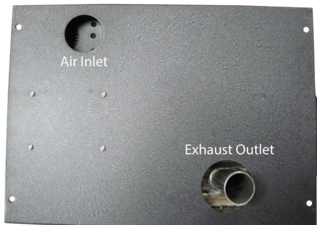
Figure 2: Bottom View of the HC Heater
