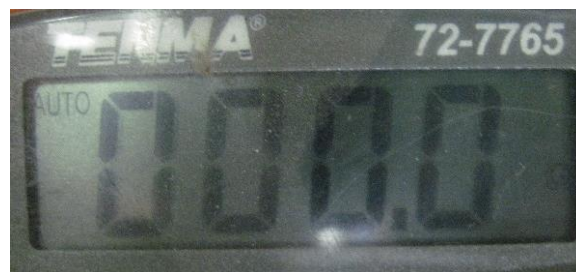
Figure 7: Digital Multi-meter Readout for New Sail Switch
