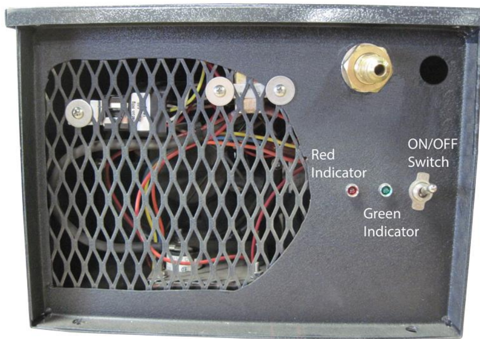
Figure 3: Side View of HC Heater (Indicator Face)
